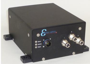
The EA -3000-H Series FSI has been specifically designed for deployment in air vehicles, but is also applicable to other platforms where size and weight are critical. It is based on the Moog Insensys OEM-3030 Fibre Sensor Interrogator family which was developed from the proven OEM-1030 of which over 1000 have been delivered, primarily for the control of wind power turbines.
