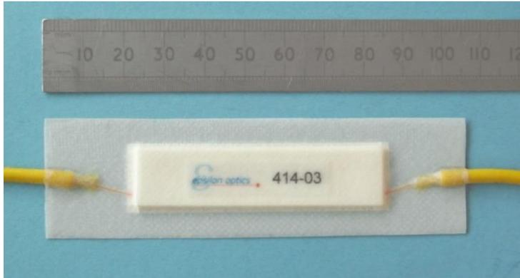
Dimensions of temperature sensor enclosure: 64 X 17 X 1.5mm
